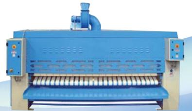
Using high-speed Image washer-extractors in combination with Image ironers improves the productivity and increases the quality. The most efficient way of removing moisture from linen is by high extraction and ironing. Our ironers are built to handle the linen direct from our washers.
