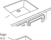
For tile, wood, or other porous materials, apply waterproof sealant around the cutout area of the countertop surface. Follow all manufacture's instructions and warnings. Allow the sealant to dry before proceeding. Use a 50/50 mixture of isopropyl alcohol and water to clean the countertop surface around the cutout area. Wipe dry with a clean cloth.
