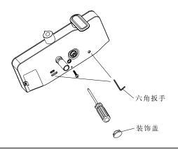
Remarks: If there is a small dimension (smaller than 10mm) difference between the faucet and the joint installation, please use a cross screwdriver to loosen (be sure not to unscrew) the screws slightly, then, screw down the screw after position adjustment.
