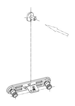
1,Please set the faucet on the joint in accordance with the figure, then, lock the fixed screw and hexagon socket from the bottom, and install the decorative cover.
