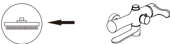
图3 Water flows out from the top shower head 头顶花洒出水
