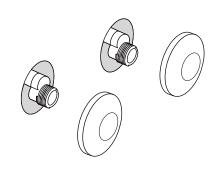
Insert washer seals into supply nuts of the faucet. Thread the faucet supply nuts onto the connectors and tighten. Connect shower hose to faucet shower outlet and hand spray. Seal provide with hose must be installed in hose inlet end.
