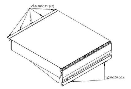
Taking into account that the height of the pit is usually 10mm greater than the height of the dock leveller, it is essential to supplement the base of the dock leveller with plates or similar to line up the dock leveller and the loading platform. The support points are indicated with arrows in the following diagram:
