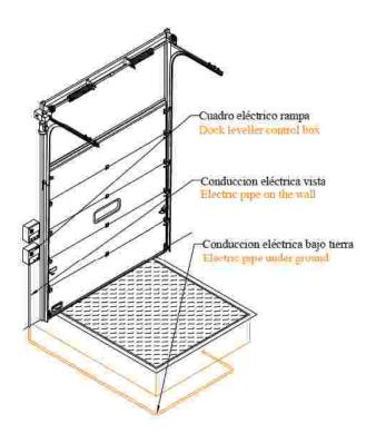
Once everything is well secured, run the cables through and connect them according to the electrical diagram found inside the control panel.
