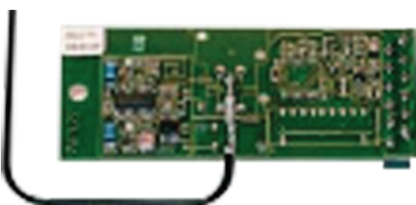
Socket for optional ELKA radio remote control receiver 434MHz, Channel 1 for complete opening Channel 2 for Partial opening
