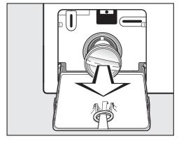
■ Remove the drain filter completely.
