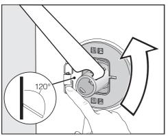
■ Push the cover out and turn the lefthand transit bar 90° using the spanner supplied.
