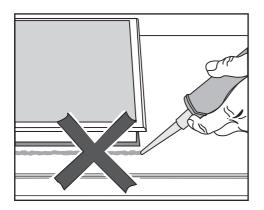
Do not use sealant between the cooktop and the worktop. This could result in damage to the cooktop or the worktop if the cooktop ever needs to be removed for servicing. The sealing strip under the edge of the top part of the appliance provides a sufficient seal for the worktop.
