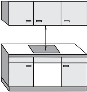
When two or more appliances are installed together below a rangehood, e.g. a gas appliance and an electric cooktop, which have different safety distances given in the installation instructions, you should select the greater distance of the two.
