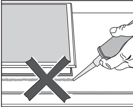
The sealing strip under the edge of the top part of the appliance provides a sufficient seal for the worktop.
