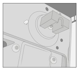
■ To ensure the microwave oven is stable, make sure that the small pin clicks into place before you reattach the feet.
