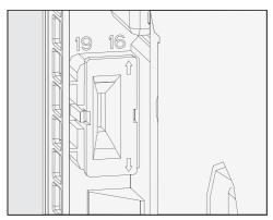
Insert the adapter so that the arrow points to the number that corresponds to the wall thickness.
