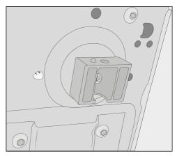
■ Unscrew the 4 appliance feet from the base of the appliance and rotate the feet a quarter turn into the raised position.
