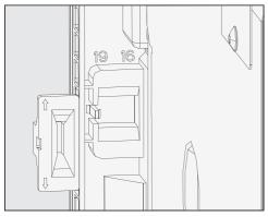
Observe the two wall thickness measurements, which can be found in the frame on the back of the appliance.
