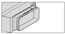
Stick the supplied sealing strip on the exhaust connection if the ducting does not sit securely up against the exhaust connection.
