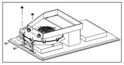
Undo the fixing brackets.
