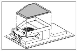
Release the 4 catches and remove the drip tray.
