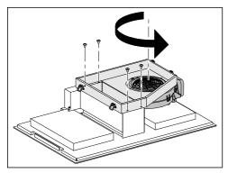
Slide the frame outwards towards the current extraction direction and tilt up to remove one side. Then slide in the opposite direction to remove the entire frame and fan. Then turn both 180°.
