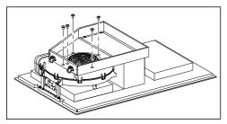
Undo the 5 screws on the fan.
