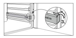
■ Then secure the FlexiClip runner to the lower rail of the shelf level (3.).
