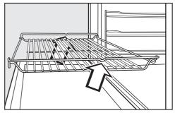
Insert the accessories into the oven with the non-tip safety notches towards the back.
