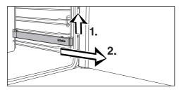
Remove the FlexiClip runner by raising it at the front (1.) then pulling it forwards along the rail of the shelf level and out (2.).
