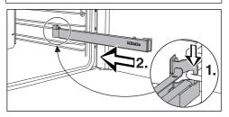
■ Hook the FlexiClip runner onto the front of the lower rail of a shelf level (1.) and then push it along the rail into the oven compartment (2.).
