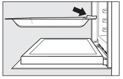
■ To remove the glass tray, lift it upwards slightly at the front when the safety notch connects with the sides of the oven.
