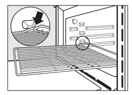
■ To remove the rack, lift it upwards slightly at the front when the safety notches connect with the sides of the oven.
