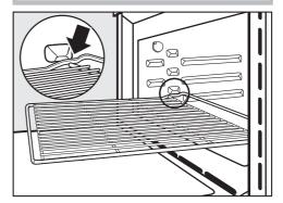
To remove the rack, lift it upwards slightly at the front when the safety notches connect with the sides of the oven.
