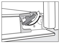
Release the locking clamps by turning them as far as they will go. The oven can be damaged if you remove the door incorrectly. Do not pull the door horizontally off
