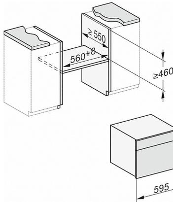
DGC7x4x, DGM7x4x, DGC7x4x, DGC7x4xX installation drawings
