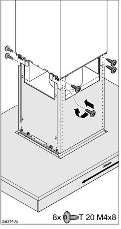
■ Raise the canopy to the desired height and secure it with the screws.
