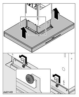
■ Hang the hood on the brackets, making sure that the controls are at the front.
