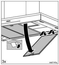
■ Remove the grease filters from the hood.
