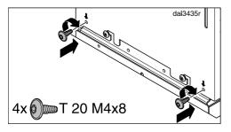
Secure the hood with the screws supplied.
