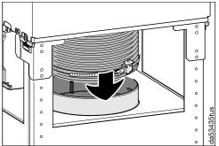
Slide the vent duct onto the vent socket and secure it (using a hose clip, for example).
