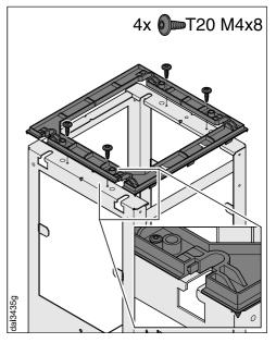
■ Mount the spacer frame onto the installation frame.
