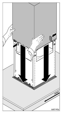
■ Hold the chimney securely, bend back the retaining tabs and carefully lower it.
