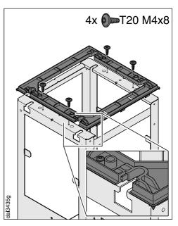
Mount the spacer frame onto the installation frame.
