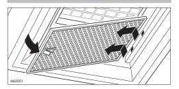
To take out a grease filter, release the locking clip on the filter, lower the filter approx. 45°, unhook it at the back and remove it.
