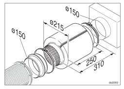
To achieve even further reductions in noise levels, a special silencer (optional accessory) can be fitted in the ducting system.
