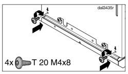
Secure the cooker hood with the screws supplied.
