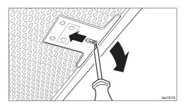
If a grease filter is inadvertently replaced upside down, insert a small screwdriver blade into the slit to disengage the clip.
