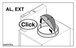
With extraction mode / external motor (AL, EXT) fit the non-return flap in the exhaust socket if your ducting system is not equipped with one.
