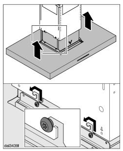
Hang the cooker hood on the brackets, making sure that the controls are at the front.
