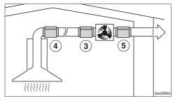
To minimise noise from the motor in the kitchen, the silencer should be positioned in front of the external motor (3) if possible, or, if the ducting is long, above the exhaust socket on the cooker hood (4). In the case of an external motor located inside the house, fitting a silencer behind the external motor (5) reduces the noise of the motor outside the house.
