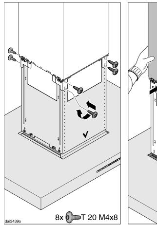
Raise the canopy to the desired height and secure it with the screws.
