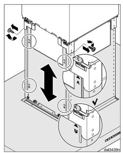
Unscrew both screws from the installation frame again.
