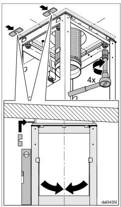
Align the installation frame with the intersecting lines and secure it with the screws.
