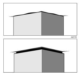
The **spacer frame** can be installed between the tower and the ceiling. This creates a shadow which gives the illusion of a gap between the ceiling and the tower. This is useful if the ceiling is not level or is uneven. The cooker hood is aligned vertically with the spacers supplied. Visual irregularities between the tower and the ceiling are then concealed by the shadow.
