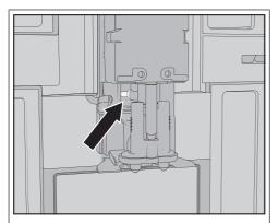
Do not remove the milk pipe connecting piece. If necessary, clean the connecting piece with the cleaning brush.
