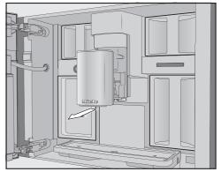
■ Pull the central spout's stainless steel cover forwards to remove it. Then clean it.
