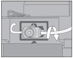
**Tip:** If necessary, turn the milk pipework towards the back at the connecting piece on the right-hand side.
