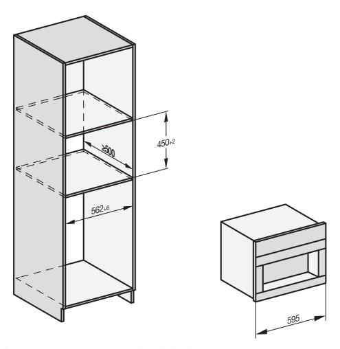
The machine can be combined with other Miele built-in appliances. In this case, there must be a full-width, closed shelf between them. If the machine it to be combined with a suitable built-in plate/food-warming drawer, no shelf is required in between.
