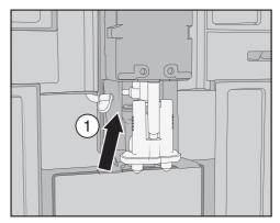
■ Detach the milk pipe from the dispensing unit as follows: pull the tab ① to the left.
