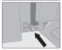
■ Remove the door opening limiters from the hinges, e.g. by prising them out with a screwdriver.
