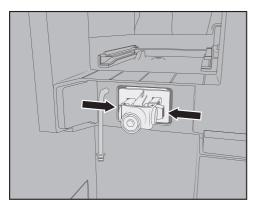
■ Press the latches on the left and right-hand sides of the milk valve holder and pull the holder forwards to remove it.
