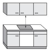
The safety distance specified by the manufacturer of the cooker hood must be maintained between the SmartLine element and the cooker hood above it.
