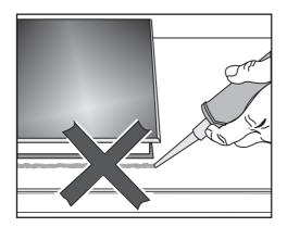
The SmartLine appliance and worktop may be damaged if the appliance needs to be removed after it has been sealed with a sealant. Do not use any sealant between the SmartLine appliance and the
