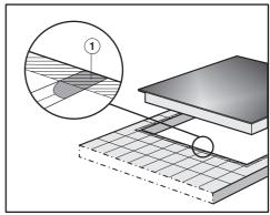
Grout lines ① and the hatched area underneath the SmartLine appliance frame must be smooth and even. If they are not, the SmartLine appliance will not sit flush with the worktop and the sealing strip underneath the top part of the appliance will not provide a good seal between the appliance and the worktop.
