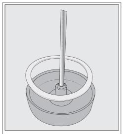
If necessary, you can remove the connecting piece and sealing ring from the milk flask lid. Once you have removed the stainless steel tube, the connecting piece is easy to push out from the inside of the lid. Clean the individual components in a dishwasher.
