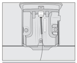
Push the cleaning brush a max. of 1 cm into the steam jet.
