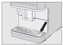
Refit the drip tray. Make sure that the drip tray cover is correctly fitted (see picture).
