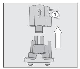
Pull off the upper silicone section with the aperture for the milk pipework ①.
