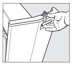
Hold the ironing table securely and pull on the release catch situated at the back of the ironing table on the right hand side.
