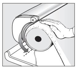
Turn the roller by hand in the direction you iron (see arrow) until the cover retaining slot is at the bottom. Switch on the ironer.
