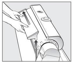
First remove the feed-in table by lifting it out of the right hand holder, and then pulling it out to the left of the roller.
