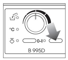
The **I-0** "On-Off" button is used for switching the ironer on and off.
