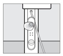
The screw-on funnel can be stored on the cable holder when not in use.
