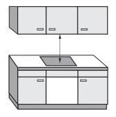
A minimum safety distance must be maintained between the ProLine appliance and the rangehood above it. See the rangehood manufacturer's operating and installation instructions for details. If the rangehood manufacturer's instructions are not available or if flammable objects are installed above the ProLine appliance (e.g. wall units, utensils rail etc.), a minimum safety distance of 600 mm must be maintained between these objects and the highest part of the ProLine appliance below.
