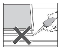
The ProLine element and the worktop may be damaged if the appliance needs to be removed after it has been sealed with a sealant. Do not use any sealant between the ProLine element and the worktop. The sealing strip under the edge of the top part of the appliance provides a sufficient seal for the worktop.
