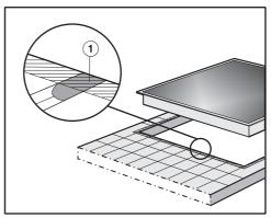
Grout lines ① and the hatched area underneath the ProLine element frame must be smooth and even. If they are not, the ProLine element will not sit flush with the worktop and the sealing strip underneath the top part of the appliance will not provide a good seal between the appliance and the worktop.
