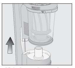
Lift the dust container upwards to remove it.
