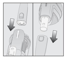
■ Slide the suction tube along the guide line on the dust container handle and down on to the PowerUnit connector from above until it audibly clicks into place (left image detail).
