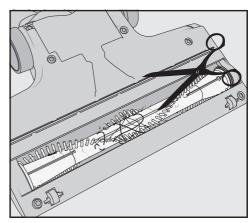
Cut any threads or hairs that have wound themselves around the roller brush with a pair of scissors. To guide the scissors, move along the guide track on the roller brush.
