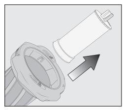
Unlock the motor protection filter by turning it anti-clockwise and lift it upwards to remove it.
