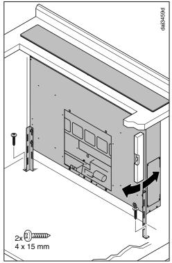
Align the downdraft extractor vertically and screw the brackets securely to the base of the housing unit.
