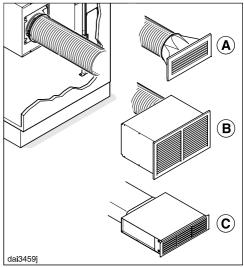
connect DUU 151 recirculation conversion kit (a) to the exhaust socket. The downdraft extractor grease filters must be fitted with DKF 22-1 charcoal filters (see "Cleaning and care")
