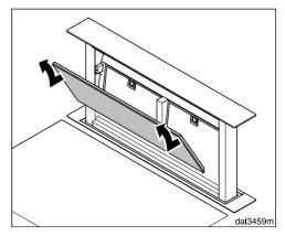
■ The panel is held in place by magnets at the top. Pull the panel forwards by the upper edge, unhook it at the bottom and remove it.
