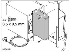
■ Secure the connection box to the downdraft extractor. It can either be fitted in the position shown or alternatively it can be fitted onto the other side of the motor, onto the back of the downdraft or onto a cabinet wall.
