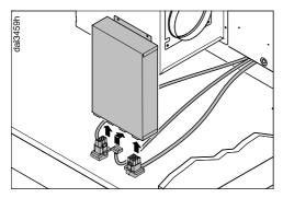
Guide the three connection leads on the bottom of the downdraft extractor through the casing and plug them into the correct sockets at the bottom of the connection box.
