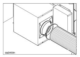
Attach the exhaust ducting, e.g. flexible hose, to the exhaust socket using a hose clip (available as an optional accessory).
