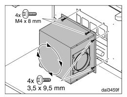
Rotate the motor so that the exhaust socket points in the required direction and secure it to the downdraft extractor.
