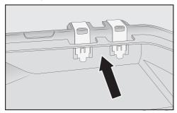
■ Clean the contacts (metal discs) and the space between them carefully, e.g. using a brush. Dry all parts thoroughly.
