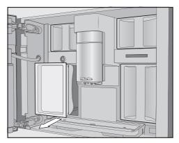
Remove the maintenance container on the left-hand side.
