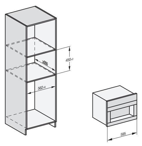
The machine can be combined with other Miele built-in appliances. In this case, there must be a full-width, closed shelf between them. If the machine is to be combined with a suitable built-in crockery/food-warming drawer, no shelf is required in between.
