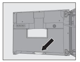
The drip tray is located at the bottom on the inside of the machine door.
