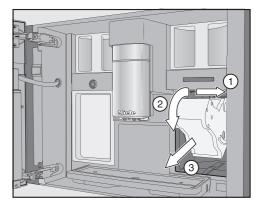
■ First, pull the brew unit sideways ① and then slide it out forwards ③. Tilt the brew unit forwards ②.
