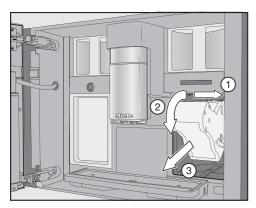
■ First, pull the brew unit sideways ① and then slide it out forwards ②. Tilt the brew unit forwards ③
