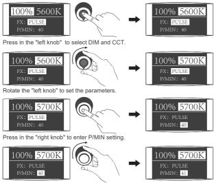
Rotate the "right knob" and set the P/MIN.
