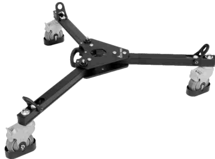
EI-7005B Video dolly Super sturdy, designed for heavy duty systems. The 100mm/4 inch wheels can be individually braked. It comes with cable guard. Folds for transporting. ⚖ 7.0kg / 15.4lbs ⌚ 100cm / 39.4in ⚖ 100kg / 220.5lbs ⌀ 100mm / 4.0in
