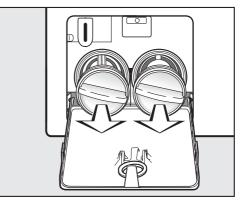
Remove the drain filters completely.
