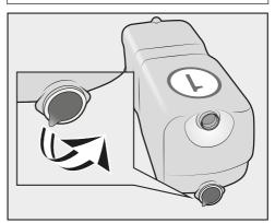
Remove the foil or the stoppers from the detergent cartridges.
