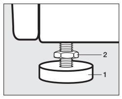
Using the spanner supplied turn counter nut 2 in a clockwise direction. Then unscrew counter nut 2 together with foot 1.
