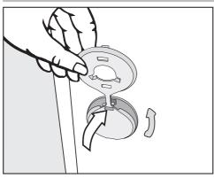
Fit the covers onto the two holes.
