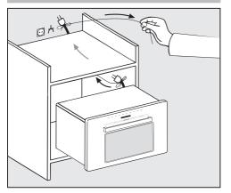
■ Slide the microwave oven into the niche. Feed the cable with the plug through the back of the unit.
