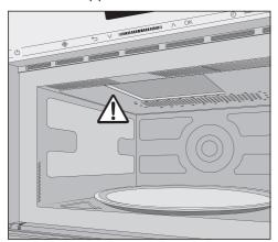
Do not remove the cover from the microwave outlet inside the oven compartment.
