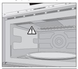
Do not remove the cover to the microwave outlet inside the oven.
