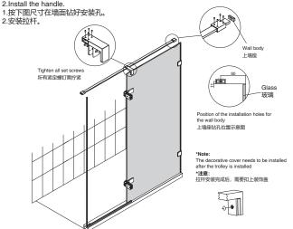
1. Loosen the lock screws on the inside of the hinge. Insert the adjusting mechanism into the opening of the glasses (make sure that the plastic cover and the plastic washers on both sides of the glasses are present before installation).Lock the hinges onto the panel glasses. Tighten the upper and the lower adjust screws while keeping the hinge horizontal. Then tighten the connecting screws on the internal cover.
