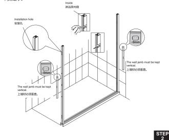
1. Check that the protective seal has been correctly installed on the bottom (see Figure B) of 1. Check that the protective seal has been correctly installed on the bottom (see Figure B) of the panel glasses and that the rubber washer is present on the inter glass jambs (see Figure A). Then insert the panel glasses into the stainless steel jambs.
