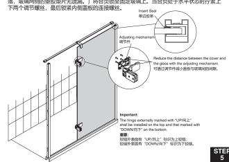
1.Adjust the closing angle with the set screw. 1.通过紧定螺钉调整好关门的角度。
