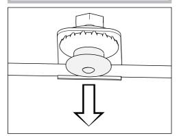
Carefully pull down the pressure cap. The top heat/grill element then lowers automatically.
