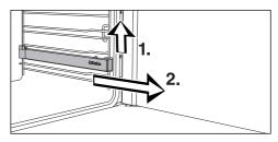
■ Remove the FlexiClip runner by raising it at the front (1.) and then pulling it forwards along the rail of the shelf level and out (2.).
