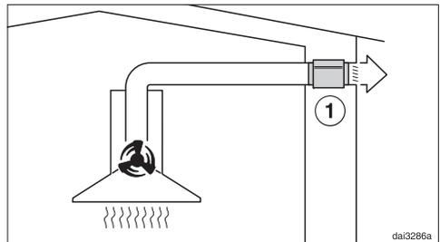
The silencer not only reduces noise from the motor outside the house, but also sounds from outside (e.g. traffic noise). For this reason the silencer must be positioned as close as possible to the ducting exit ①.
