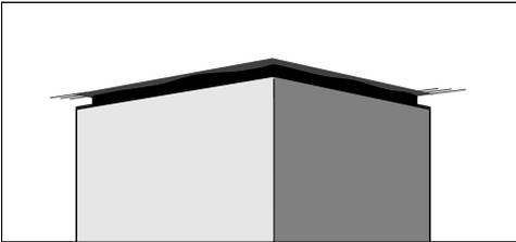
The **spacer frame** can be installed between the tower and the ceiling. This creates a shadow which gives the illusion of a gap between the ceiling and the tower. This is useful if the ceiling is not level or is uneven. The cooker hood is aligned vertically with the spacers supplied. Visual irregularities between the tower and the ceiling are then concealed by the shadow.
