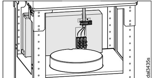
The strain relief must be used to ensure problem-free connection.
