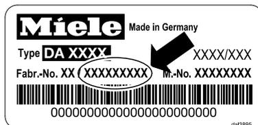
The password for your cooker hood consists of the last 9 digits of the serial number. This can be found on the appliance's data plate.
