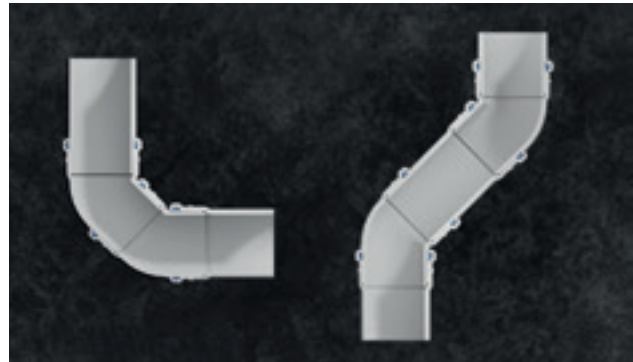
Fig. 20: Changes of direction with 45° bend.
