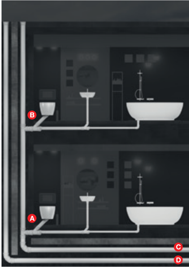
Fig. 11: Minimum fall for waste water pipes, example.
