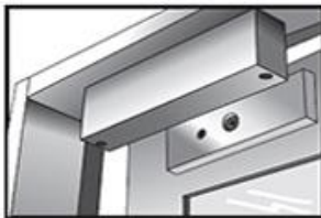
Regular Installation (outswing door)
