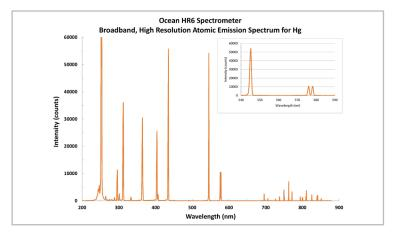
The Ocean HR6 provides broadband, high resolution performance for emission and other measurements.
