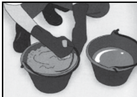
1. Tile adhesive with water portion adhesive:water 4:1
