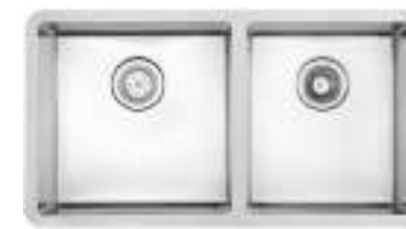
Blade 27112 Silky Finish Bowl size : 1-400mm x 400mm x 200mm 1-340mm x 400mm x 200mm Overall dimensions : 825mm x 450mm Thickness : 1mm
