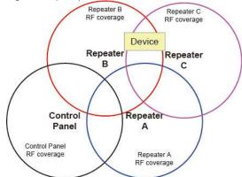
From the displayed diagram, the device is located between the RF coverage areas of Repeater B and C. Users can choose to learn the device into Repeater B only, learn into Repeater C only, or learn into both Repeaters B and C.
