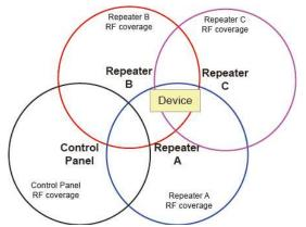
From the displayed diagram, the device is located between the RF coverage areas of Repeater A, B and C. Users can choose to learn the device into Repeater A only, learn into Repeater B only, learn into Repeater C only, or learn into Repeaters A, B and C. It is **recommended** to learn the device into Repeater A only or Repeater B only (and not to Repeater C) to reduce signal traffic.
