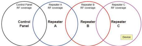
Repeater C must be learnt into Repeater B. Do not learn Repeater B into Repeater C. Repeater B must be learnt into Repeater A. Do not learn Repeater A into Repeater B. Repeater A must be learnt into the Control Panel.
