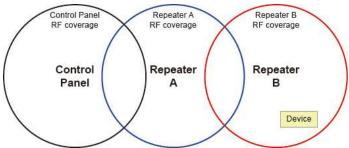
The device is closest to Repeater B, and is therefore learnt into Repeater B but not into Repeater A.
