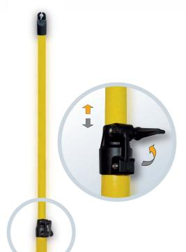
Telescopic pole with two sections made of reinforced fibreglass tube  $\emptyset$  40 and 32 mm with humidity-proof seals on each end, hand protector, grip, tip and M (Metric-10), U (Universal), B (Bayonet) or P (Hexagonal + Metric-10) head.
