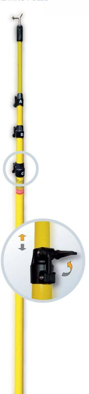
Telescopic multiple section pole made of reinforced fibreglass tube with variable circular shape that allows to wedge automatically each section. The upper section is filled in with foam according to IEC 60855.
