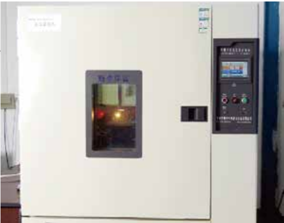
High-low temperature test of the aircraft platform
