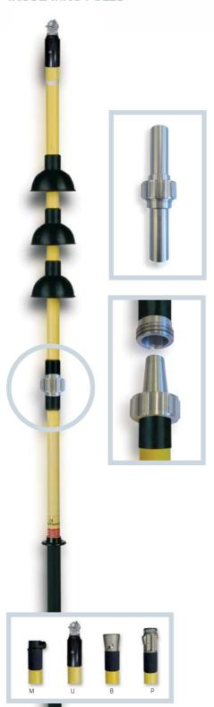
Connectable pole with two or three sections made with polyester and fibreglass tube  $\varnothing$  40 mm with hand protector, grip, tip, 3 deflecting hoods and M (Metric-10), U (Universal), B (Bayonet) or P (Hexagonal
