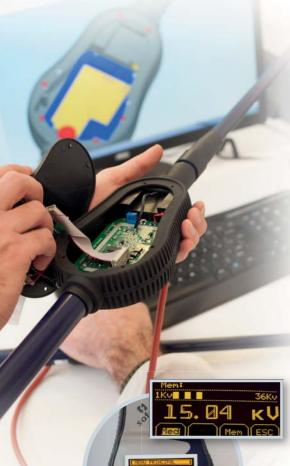
Bipolar voltage detector with digital display OLED to be used in MV netwoorks.
