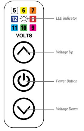
LED Indicator: Single blink = Whole Value Double blink = Half Increment Ex. Solid green indicates 10V Flashing green indicates 10.5V Battery Level Check: Press and hold power button
