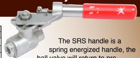
The SRS handle is a spring energized handle, the ball valve will return to pre-determined closed (or open) position when an operator disengages from handle, provides safe and positive fail close or open operation, creating a reliable sampling, filling, dispensing, and pressure relief valve. Full S.S. construction provides excellent corrosion resistance for extended service life.
